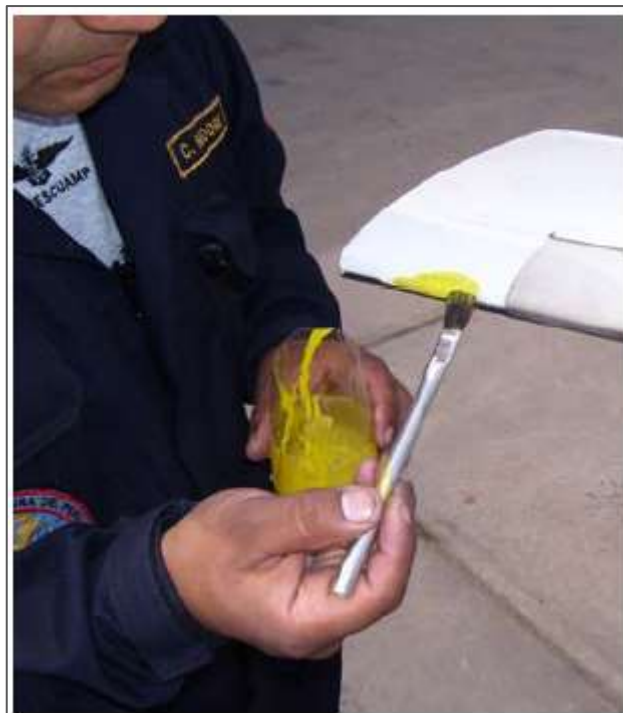
Figure 2. Primer applied to exposed area
