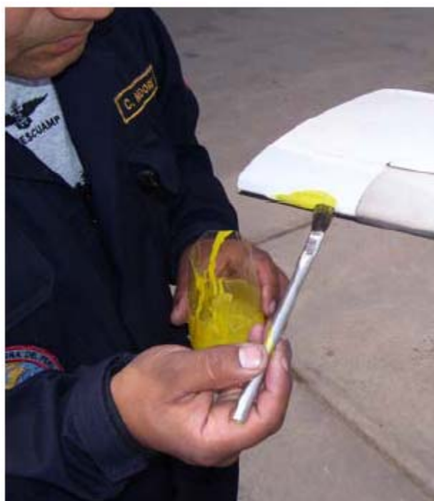
Figure 2. Primer Applied to Exposed Area
