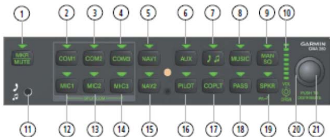
Figure 7-3. GMA 350H Controls
