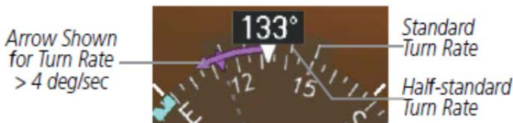
Figure 2-23. Turn Rate Indicator and Trend Vector Bearing Pointers and Information Windows
