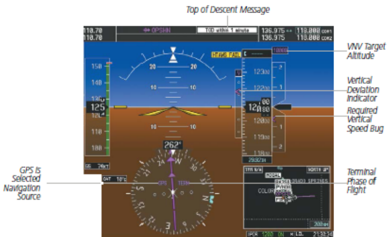
Figure 2-33. Vertical Navigation Indications (PFD)
