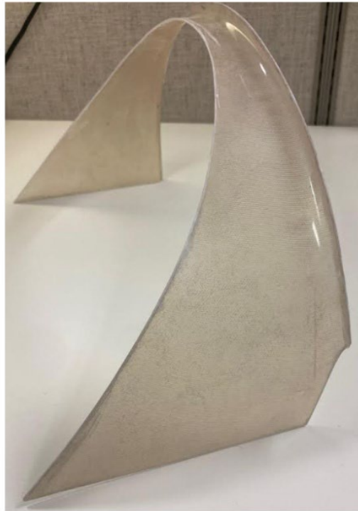
Figure 4. Finished appearance of modified pulley shroud flange; shown unpainted and uninstalled
