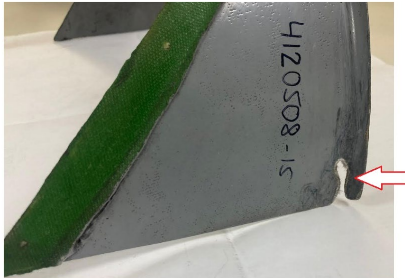
Figure 2. Wear damage to flange (Flange shown disassembled from pulley shroud assembly)
