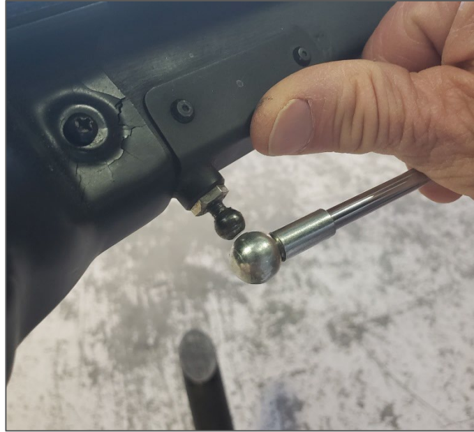
Figure 4. Pull gas spring off ball (both ends)
