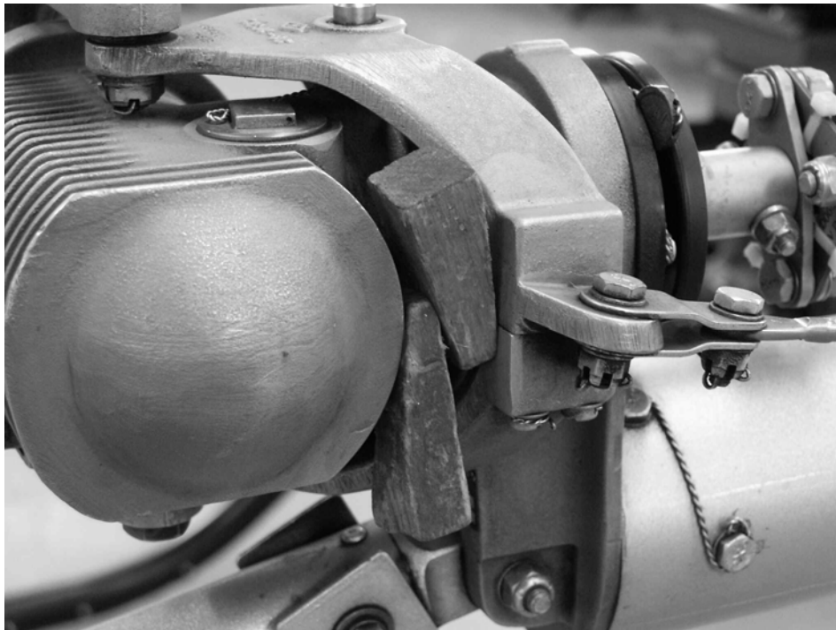
WOODEN WEDGES INSTALLED
