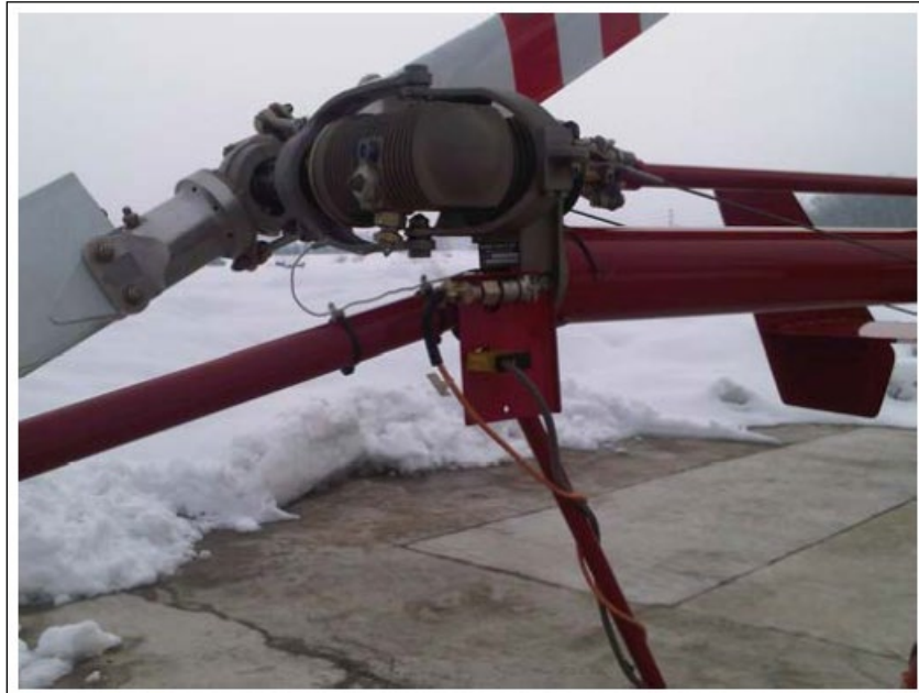
Figure 9-34.1. Velocimeter and T-0152 Installation
