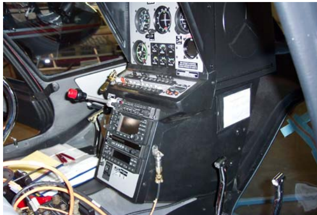
Figure 3. Velocimeter installed on the lower instrument panel (280FX shown).
