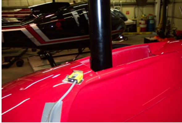
Figure 2. Optical Sensor installed on 280FX air scoop.
