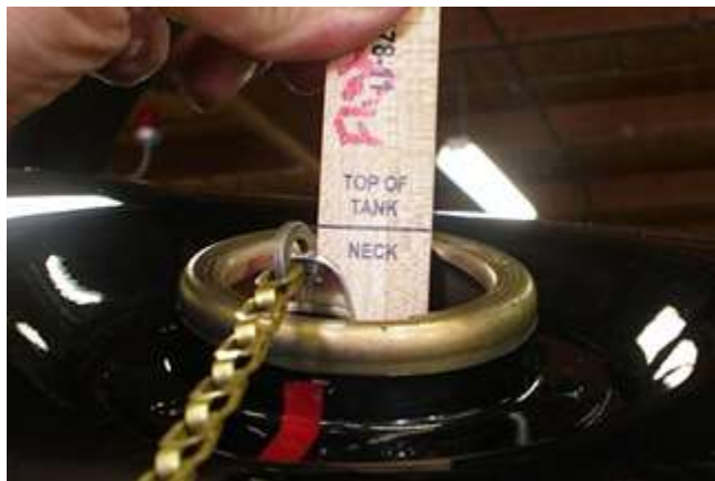
Figure 1. Proper placement of the fuel dipstick. The TOP OF TANK/NECK line is at the level of the top of the fuel tank.
