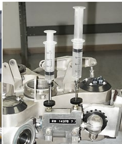
(Servicing the dampers using Tool T-2896 is shown in the photo to the right.)
