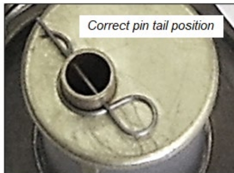
Figure 13-21.1a. Correct Installation of Pin; Curved tail is installed under the straight tail.
