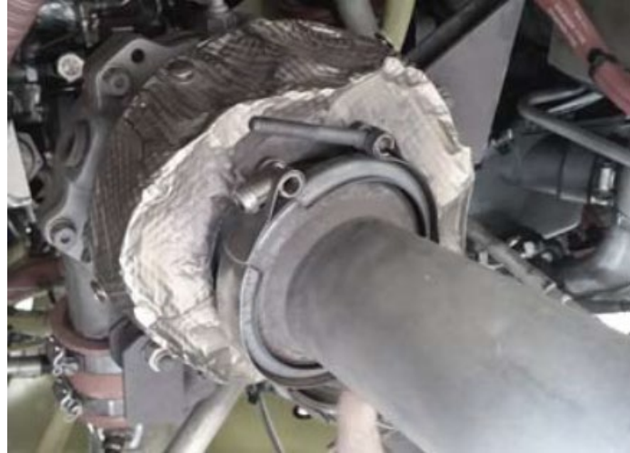
Figure 13-8.5. V-band coupling(1), P/N LW-13464, positioned for ease of spot weld inspections
