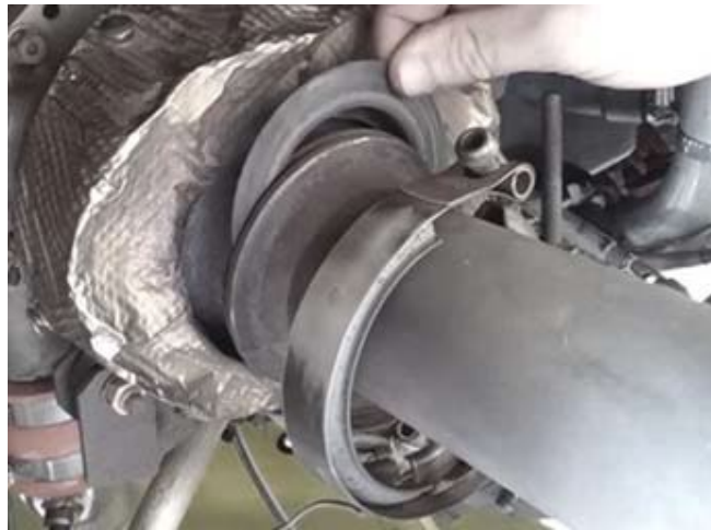
Figure 13-8.3. Installing metal gasket, P/N LW-14485
