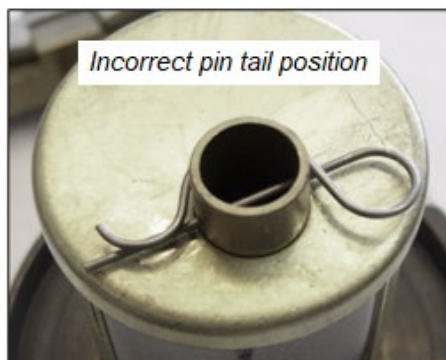
Figure 13-21.1b. Incorrect Installation of Pin; Curved tail is installed over the straight tail.
