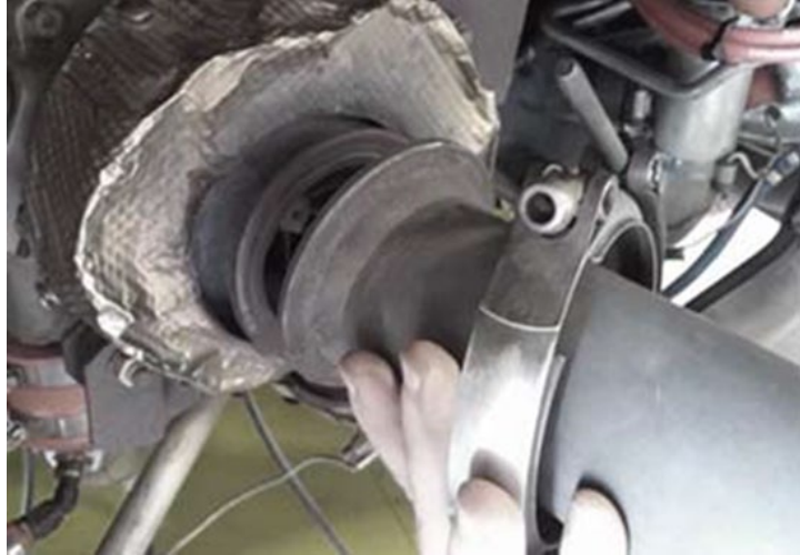
Figure 13-8.2. V-band coupling (1), P/N LW-13464, joining the tailpipe to the turbocharger exhaust outlet
