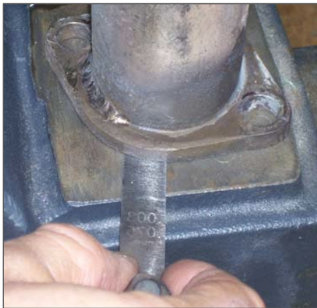
c) .001" Feeler Gauge Inserted
