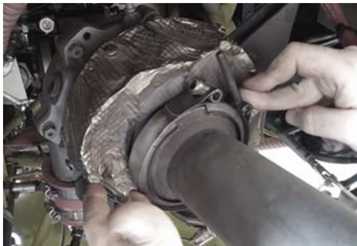
Figure 13-8.4. Flanges and metal gasket joined; V-band coupling positioned over joint
