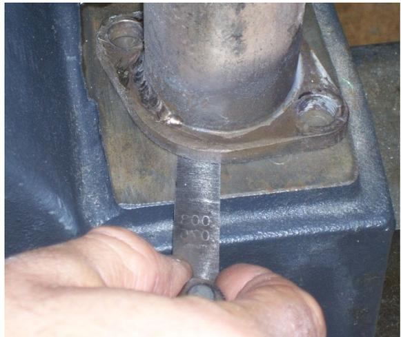
13. A large punch and hammer can be used to tap the flange against the flat surface of the vise to straighten the flange. The stainless steel is quite soft and can normally be re-shaped to repair the warpage.
