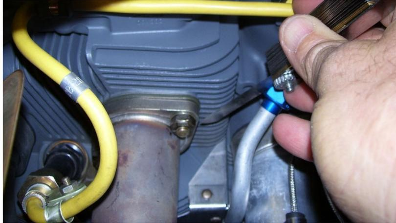
8. if the feeler gauge can be inserted between the exhaust port and the exhaust pipe on the back side, but not on the near side, then the #4 exhaust stack is too long and is preventing the exhaust pipe from sealing against the exhaust port.
