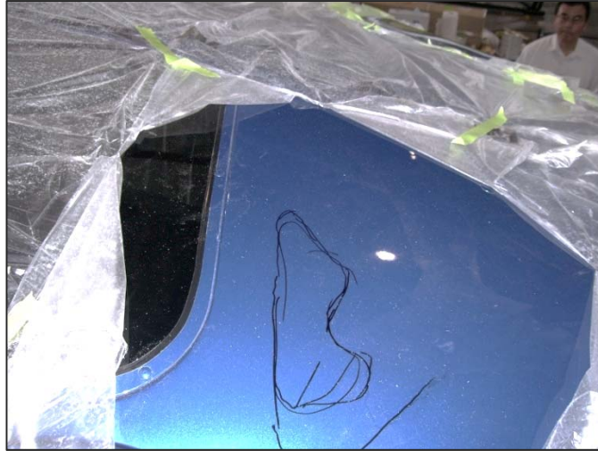
Figure 1. Repair area outline marked
