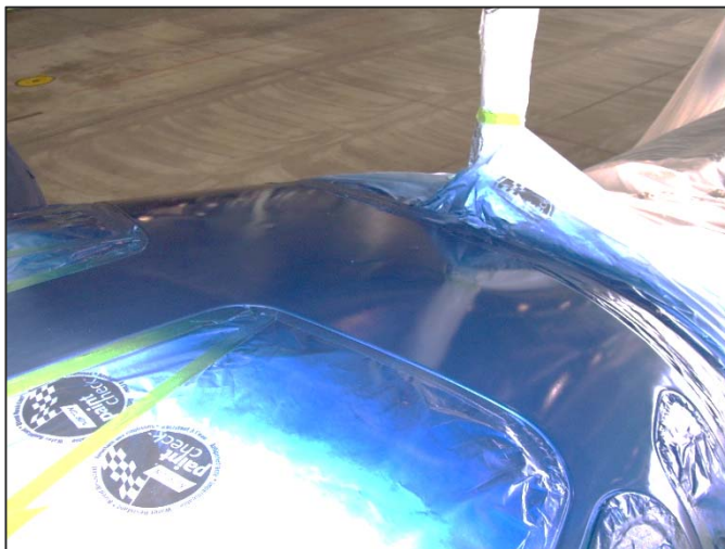
Figure 6. Repair area repainted
