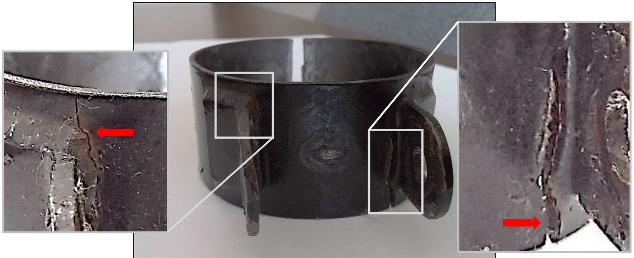
Figure 8-8.1 Cross Tube Weldment Clamp Cracks
