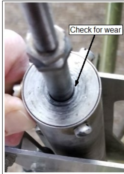
Figure 11-3.1 Spring Capsule Wear Inspection Area
