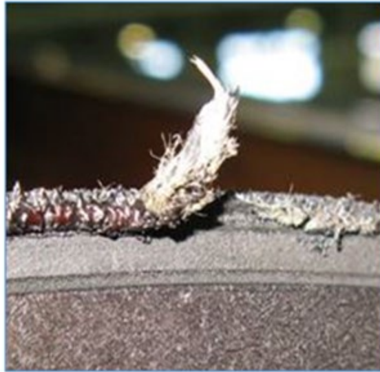
Figure 11-8.9. Drive Belt Visual Inspection – Cord Tail
