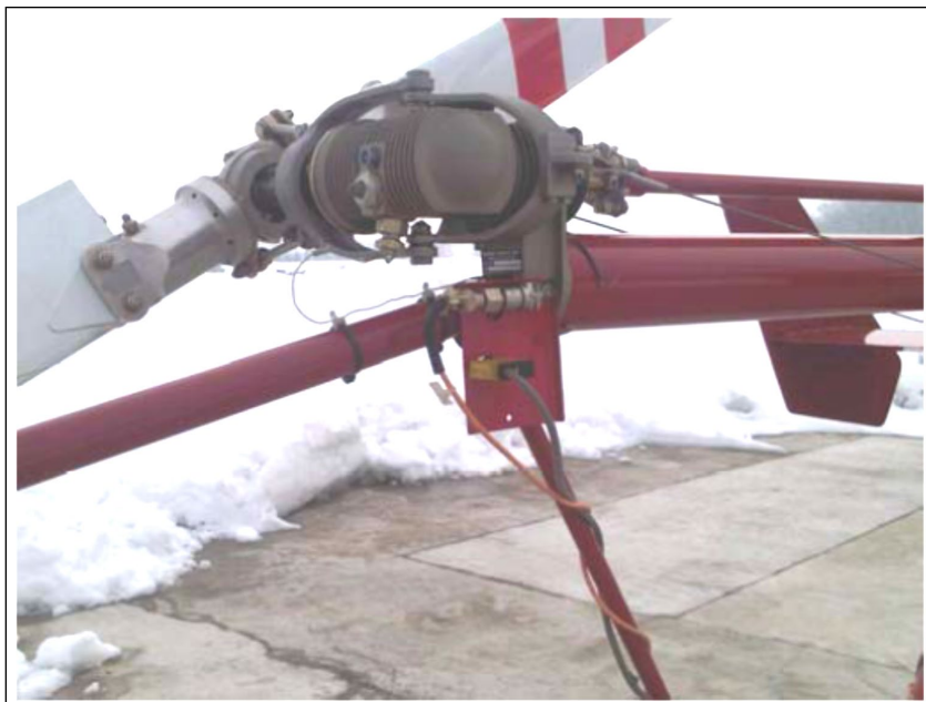
Figure 10-8. Velocimeter and T-0152 Installation
