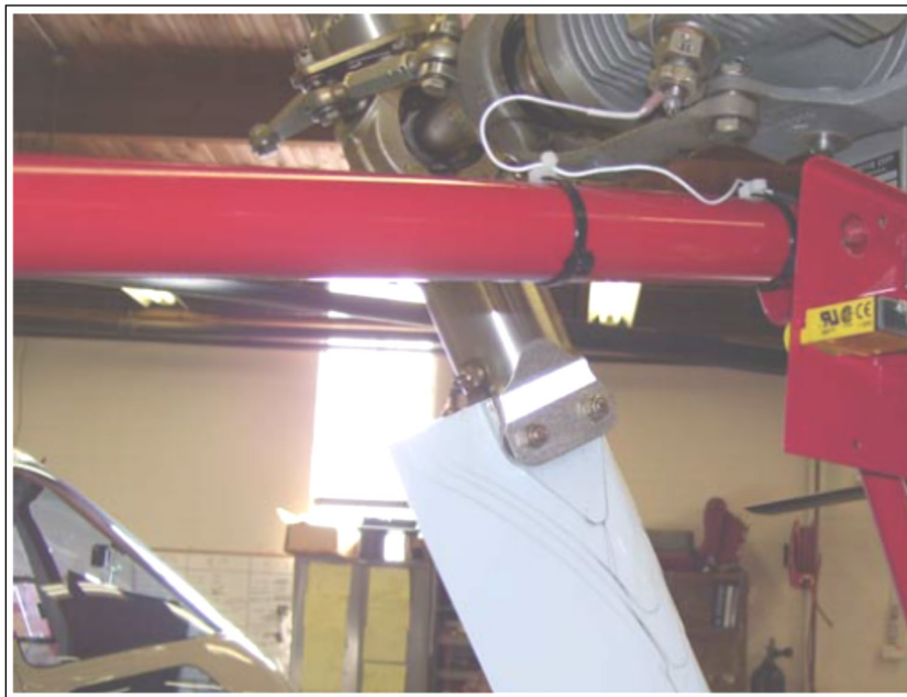
Figure 10-9. Reflective Tape Installed on the Target Blade
