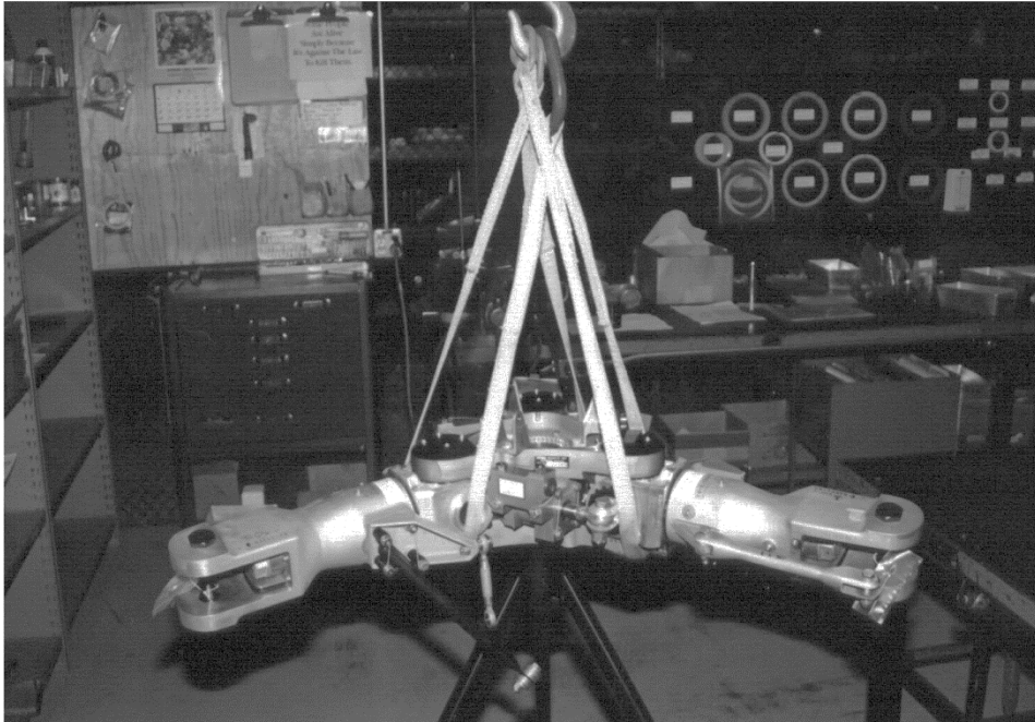
Lifting Sling Installation
