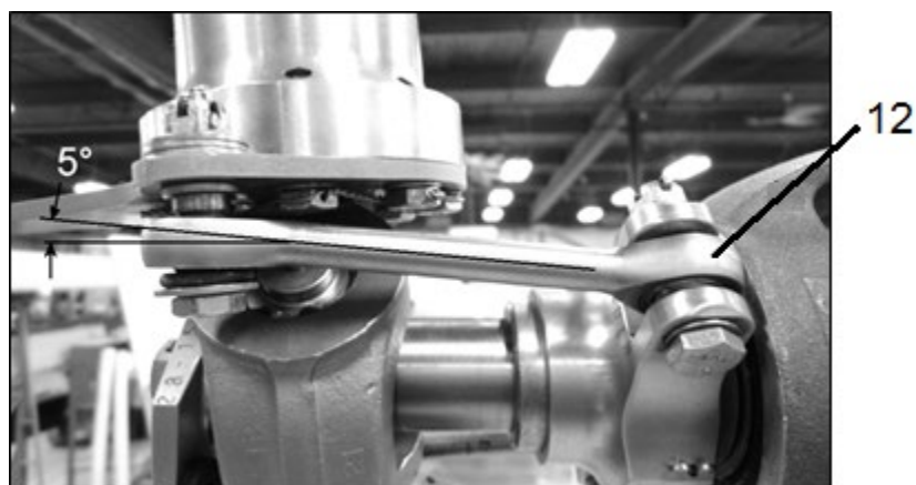
Figure 10-4. Pitch Change Link Installation
