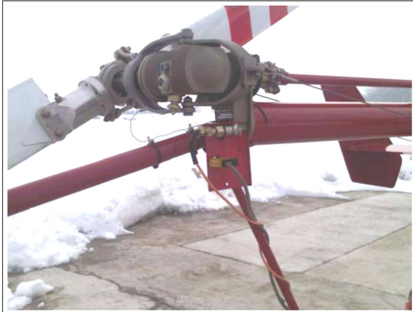
Figure 10-8. Velocimeter and T-0152 Installation
