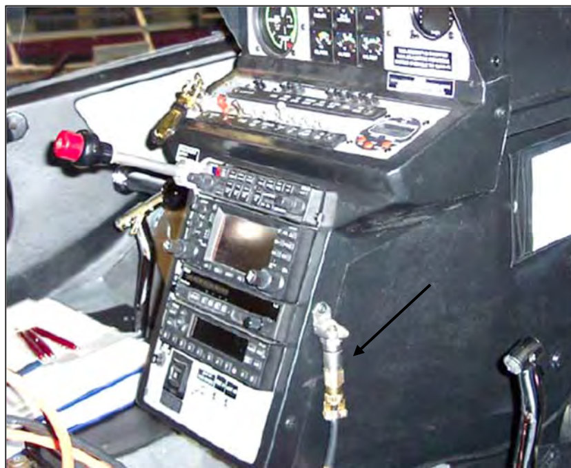
Figure 12-3. Velocimeter Installation (280FX)
