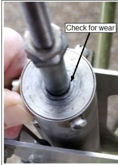
Figure 11-3.1 Spring Capsule Wear Inspection Area
