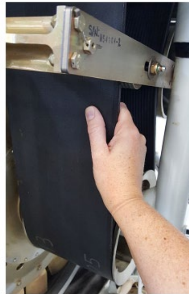
Improper Method – DO NOT grip edge of belt
