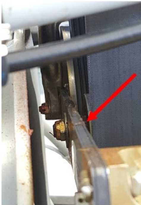
Inspection point – Center pulley, forward edge
