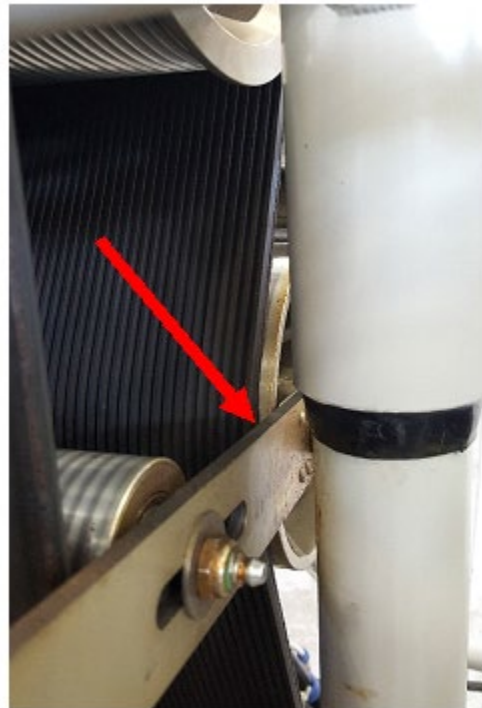
Inspection point – Center pulley, aft edge
