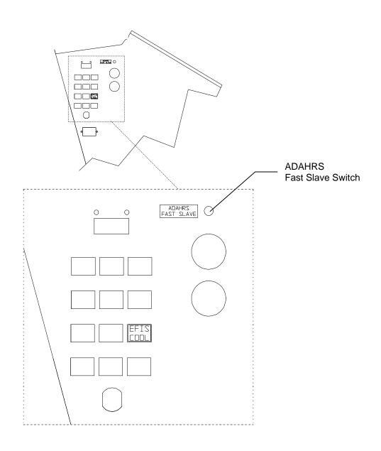
Figure 5-8. Fuse Panel and Fast Slave Switch Location
