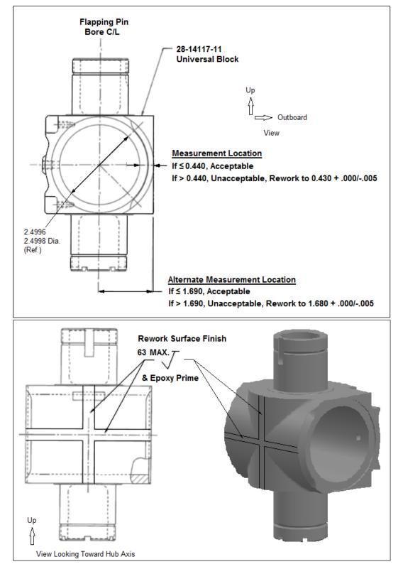
Figure 1. Universal Block Inspection (top); Rework Criteria (top and bottom)
