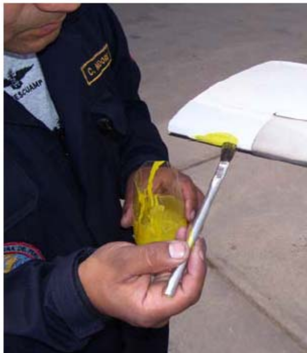
Figure 2. Primer Applied to Exposed Area
