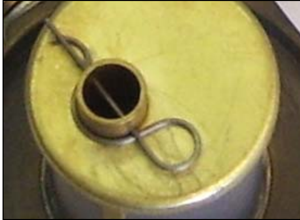
Figure 1. Correct Installation of Pin; Curved tail is installed under the straight tail.
