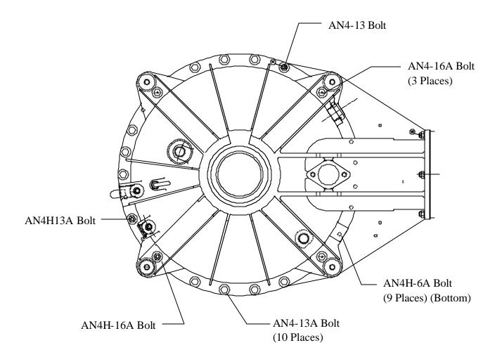
Figure 1. Main Rotor Gearbox Attachment Bolts
