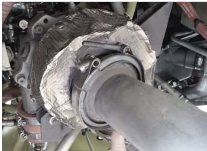
Figure 5d. Clamp positioned for ease of spot weld inspections
