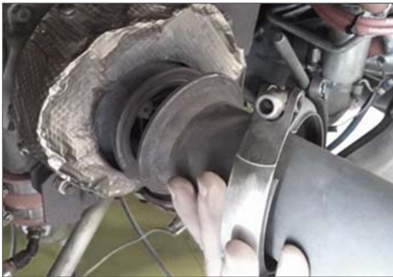
Figure 5a. Clamp P/N LW-13464 prepared for joining the tailpipe to the turbocharger outlet
