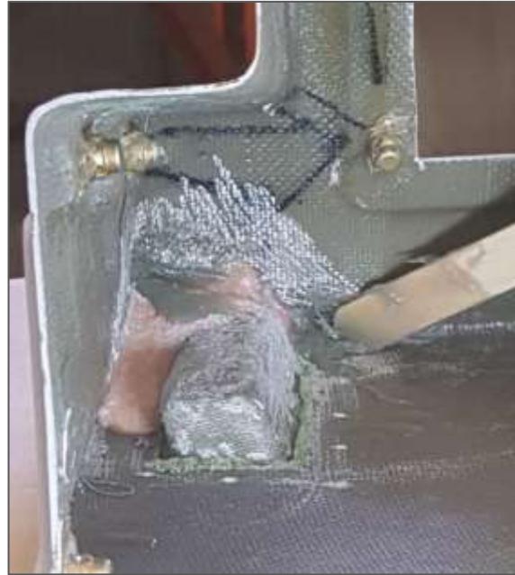
Figure 5. Fillet putty/DDM-9 MEKP mixture applied to material and inner hand hold
