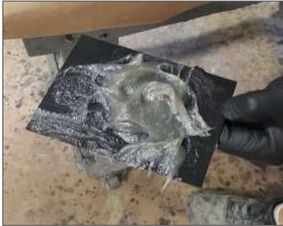
Figure 5. Fillet putty/DDM-9 MEKP mixture applied to material and inner hand hold
