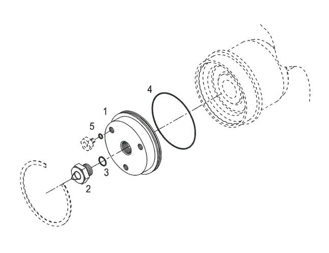
Figure 1. ORC Cover Equipped with Sight Plug
