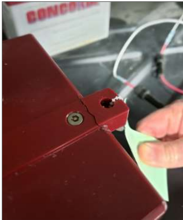
Figure 1. Cracked battery mounting tab
