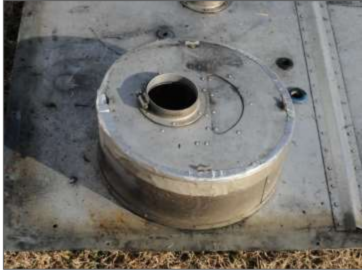
Figure 3. A Model air filter container assembly
