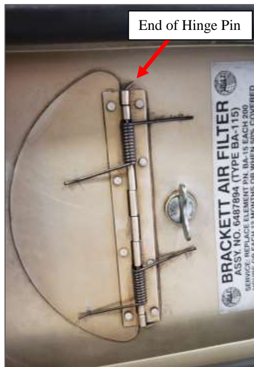
Figure 4. Backfire door hinge pin (Modified)
