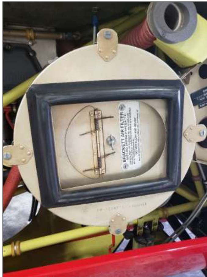
Figure 2. Air filter container assembly
