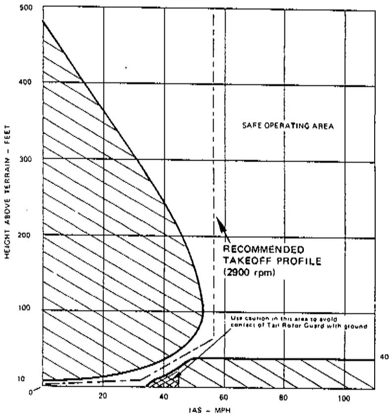
Weight applicability of H-V Diagram is based on hover capability at 3.5 feet skid height. (Reference FM 5-3.)
