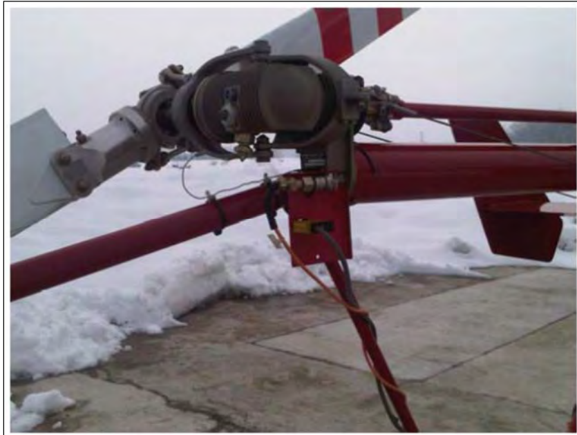
Figure 9-34.1. Velocimeter and T-0152 Installation
