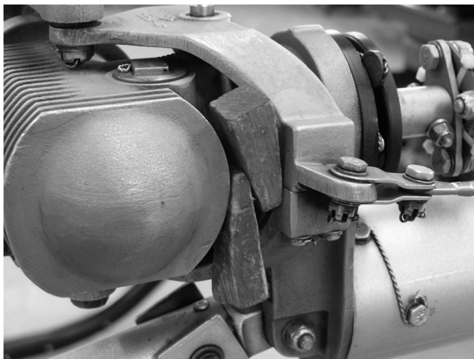
WOODEN WEDGES INSTALLED
