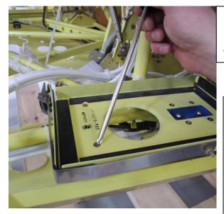
6. Remove four battery tray mounting screws. Remove tray from aircraft.
