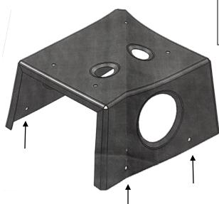
11. Install speed control mount in tray using four screws P/N: AN525-10R10, with locking nuts P/N: MS21044N3, and washers P/N: AN960-10L. Screw should have protrusion of at least two threads. Shim as required using washer P/N: AN960-10 or AN960-10L
