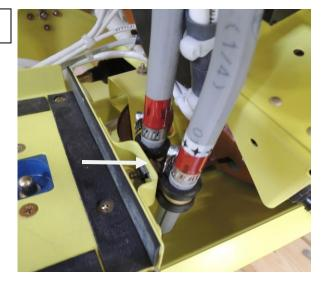
5. Remove tie down bracket with associated hardware.
