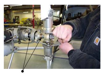
2. Using the tail rotor retention plates operate the slider mechanism in and out.
