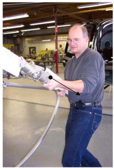
These tests should isolate what is causing the 'dead spot' in the tail rotor and assist the mechanic in determining what parts need to be replaced without needlessly replacing airworthy parts.
