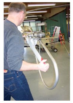
Then, pushing on tip of the blade with one hand, use your other hand to rotate the blade, feeling for roughness in the bearing. This test sideloads the roller bearings and checks their condition.
