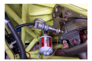
Magnetic Pick-up installed on 480 Swashplate.
