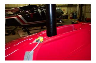
Optical Sensor installed on 280FX air scoop. Mount the bracket under the fuel tank mounting screws on F 28 series helicopters.
