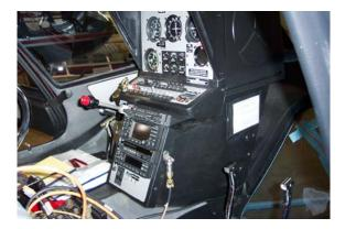
Velocimeter installed on 280FX lower instrument panel
