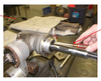
3. Remove the retaining ring, [N50000-175], from the output shaft seal. Using an awl or a small screw driver, carefully remove the seal, [9276]. NOTE: Note the part number on the seal. Use the same part number to replace seal.
