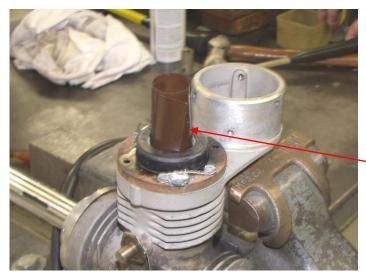
6. Clean the tail rotor transmission seal surface and the O.D. of the new seal with cleaner/ primer, or other suitable solvent. Apply a small amount of Loctite-277, Red sealant to the seal and lubricate [STP and oil mixture], the seal lip and install the seal. Use shim stock wrapped around the input nut to protect the seal lip during installing. Use a soft mallet, and a drift to tap in seal
