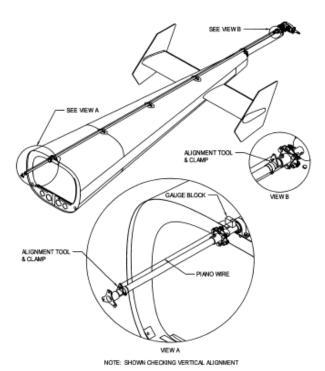
Figure 11-13. Tail Rotor Drive Shaft Alignment
