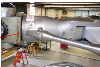
Be sure to remove the purge plugs from the grip when greasing the grip to prevent the seal from being pushed out from the grip. Use only Shell 22 (Recommended) or Mobil 28 in Grips.
