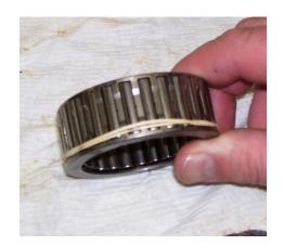
J. Wrap the sprag assembly with a small rubber band and slide it over to the edge of the assembly closest to the arrow etched on the end race.
