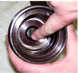
D. Remove the top bearing (ECD4016) and the (4151005–( )) shims from the bearing and sprag assembly.
