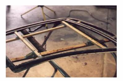
Lay the door frame on saw horses, and lay the glass on top. Mask off the areas not to be glued or painted.
