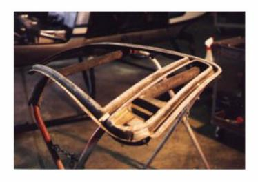
Remove the old glass, and the abrasion strip from the fiberglass frame.
