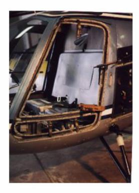
Clamp the frame back in the door opening so that it fits the cabin shape. If it is really warped, it can be repaired by cutting slots in the frame until it relaxes and then repairing it with some fiberglass.
