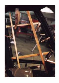
The next step is to attatch a "ladder back" to the door frame while it is clamped in the door opening.
