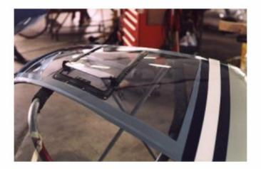
Bond the glass to the frame using one of the flexible adhesives, such as PRC or Scotch 801. Use enough clamps to evenly distribute the clamping pressure.
