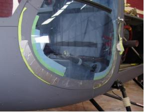
Normal fiberglass refinishing procedures can now be used to re-finish the inside door frame channel. Kyron Black Semi-gloss spray paint does an excellent job refinishing the inner door frame and matching the original color.
