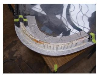
6. Mask off the acrylic glass, the outside painted surface of the door, and the door sill of the cabin to prevent contamination by the resin. Lay up three layers of 6 ounce bidirectional fiberglass cloth over the area of the door frame channel that was sliced. Install the door back onto the helicopter while the fiberglass is still wet and tape the door to the cabin to help hold the shape while the resin cures.
