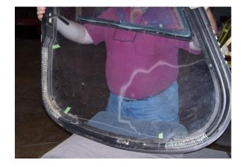
4. Use a heat gun to gently heat the outside areas of the door in the areas that were cut to reshape the door to the cabin. Start by holding the heat gun about 8 inches from the surface of the door and slowly move it in a circular pattern while moving it closer to the door; to warm the acrylic slowly and prevent over heating it.
