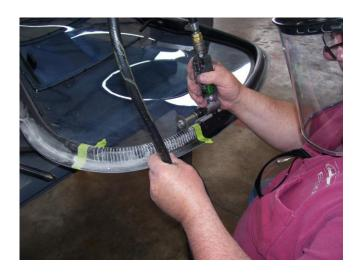
3. In most cases the door will need to be reshaped in two places, in the font and aft corners of the door.
