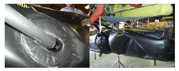
Figure 6. Drag Strut Inserted Through Float Cell Hole
