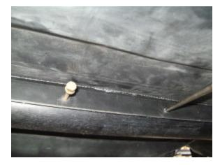
Figure 8. Attachment of Float Girt to Skid Tube
