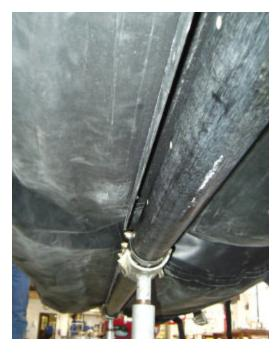
Figure 7. Float Flanges Aligned With Skid Tube
