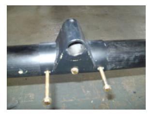
Figure 2. Wheel Bracket Removal
