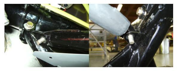
Figure 4. Drag Strut Removal
