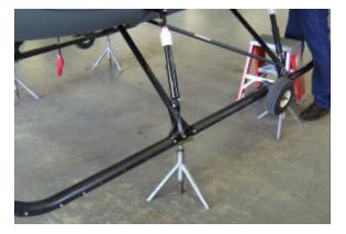
Figure 1. Stands Under Landing Gear
