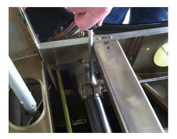
NOTE: Isopropyl Alcohol is an effective cleaner to use. Do not use brake cleaners as they will leave a residue, causing the lock to slip.
