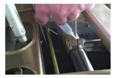
3. Using clean compressed air, blow between the friction lock and the collective tube while moving the collective up and down a few more times.
