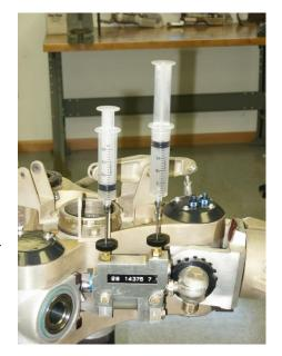
If you have to bleed dampers more than once in 50 hours, (the exception is a ship that is doing a lot of autos) there is a rule of thumb as to whether to repair or to overhaul.
