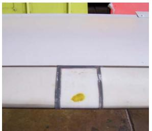
masking tape to allow the sealant to flow to a nice tapered edge. DP190 will gel in 90 minutes at 72° and full cure will be achieved in about 8 hours. It will cure faster in warmer temperatures and slower in colder temperatures.
