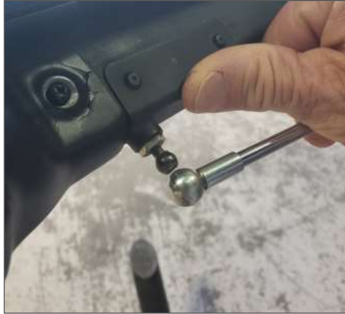
Figure 4. Pull gas spring off ball (both ends)
