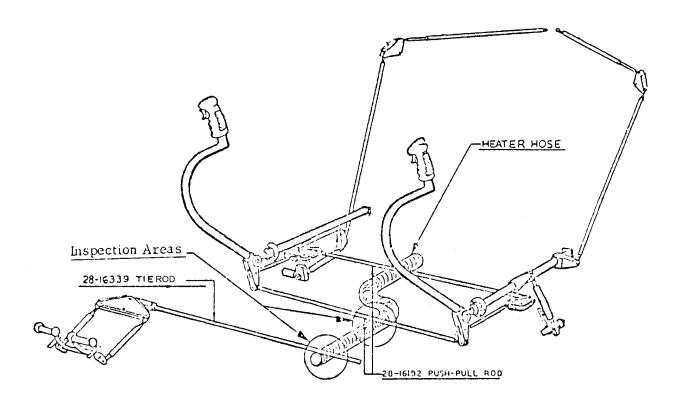
Any wear on the aluminum control rods exceeding .015 depth should warrant replacement. Extra clamping may he required to obtain clearance between the heater hose and the push-pull control rods. Normal clearance is about .38 in.
