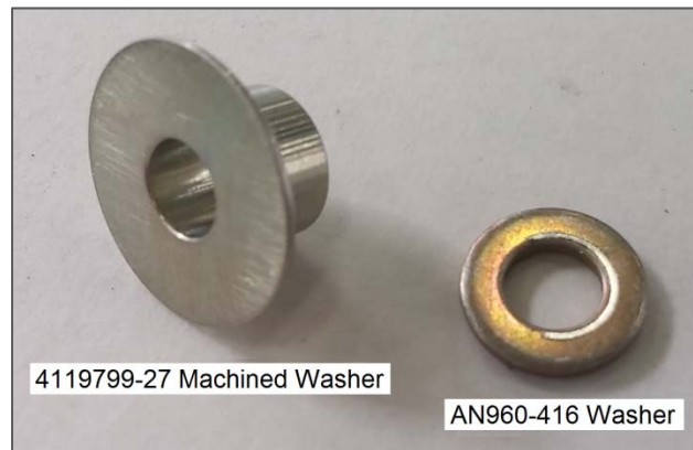
Figure 1. Machined Washer 4119799-27 (Left), Washer AN960-416 (Right)
