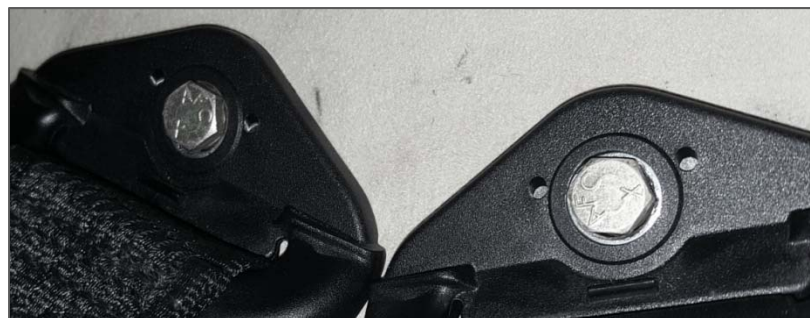
Figure 3. Incorrect Washer Installation – Machined Washer Installed Behind the Restraint
