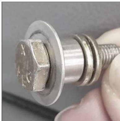
Figure 4. Bolt, Machined Washer, Shoulder Harness Attachment (not shown), and Washers Stack Up (shown without threadlocker)
