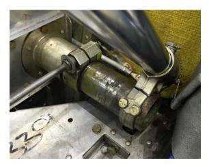
It was reported that a technician found a cracked pilot's collective socket (P/N 28-16186-1) on a F28-C helicopter. The time and history of the helicopter is not known. Enstrom recommends inspecting the collective mounts carefully during scheduled inspections or any time the collective cover is removed.
