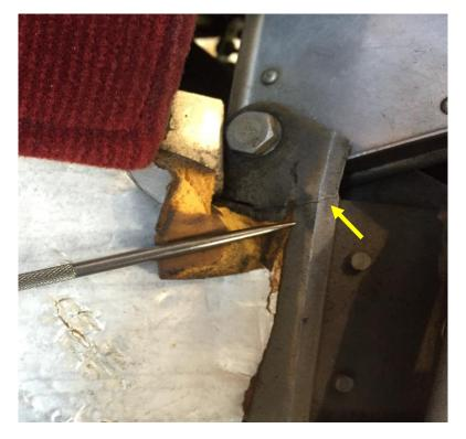
It was reported that a technician found a cracked pilot's side cabin cyclic bell crank mount (P/N 28-11307-1) on a 280C helicopter. Enstrom recommends inspecting both co-pilots, and pilot's side mounts carefully during scheduled inspections or any time the seat deck is removed.
