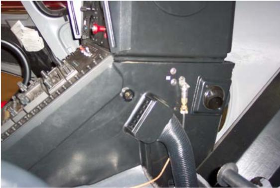
Velocimeter installed on 480 lower instrument panel.
