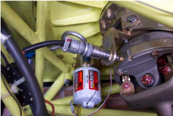
Magnetic Pick-up installed on 480 Swashplate.
