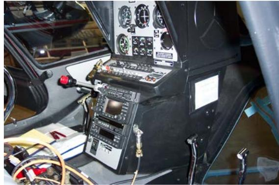
Velocimeter installed on 280FX lower instrument panel
