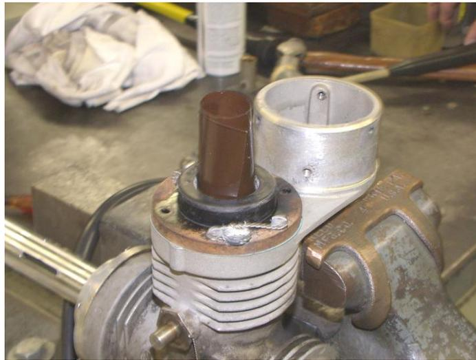
17. Install the retaining ring (15) or the tab washers if used.
