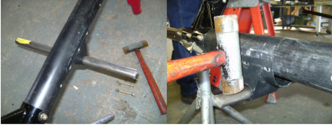
Figure 3. Bracket Removal
