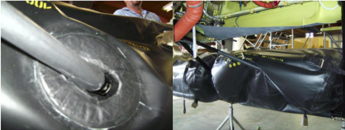
Figure 6. Drag Strut Inserted Through Float Cell Hole
