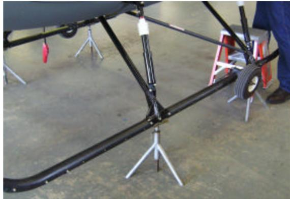
Figure 1. Stands Under Landing Gear
