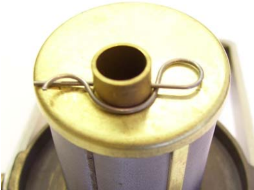
Figure 2 Incorrect installation; tail of pin is installed overtop of straight section.
