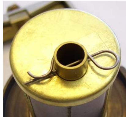
Figure 3 Incorrect installation; curved section of pin is installed overtop of straight section.
