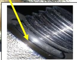
*Tapered rod end shoulder is below the surface of the dogleg. ACTION: **Torque nut and install cotter pin.***
