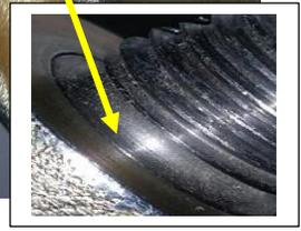
*Tapered rod end shoulder is flush with the surface of the dogleg. ACTION: **Torque nut and install cotter pin.***
